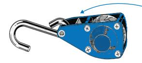
Ease tension while pulling the release clip.
