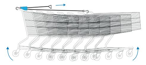
3 Engage the C3 ST Safety Rope by pulling the rope through the ratchet with moderate force to create lift. **Do not over tighten.**
